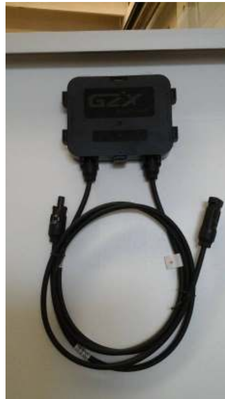
Figure 5: Detail view of cables, connections and Polarity mark on the cable
